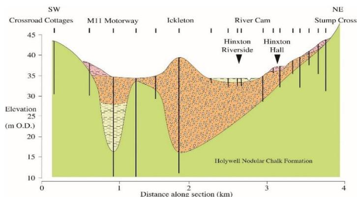
because of the unusual geological configuration of the Ickleton/Hinxton area. The diagram shows a NE to SW section drawn from Stump Cross, through Hinxton Hall (on the Genome Campus) to just beyond the M11, derived from borehole records.<sup>1</sup>
