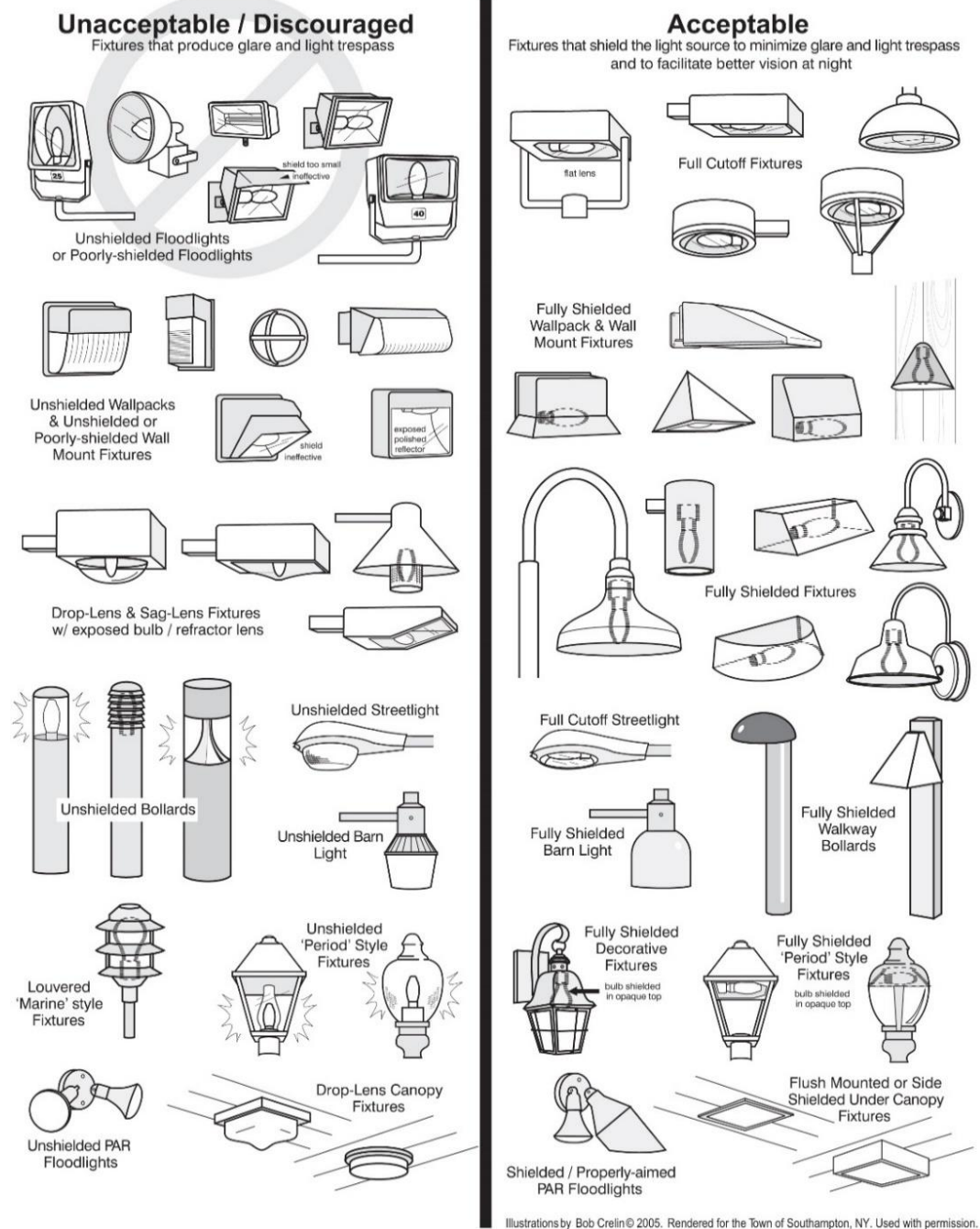
Figure 2—1 - Example of luminaire types approved by the IDA - (Source IDA)
